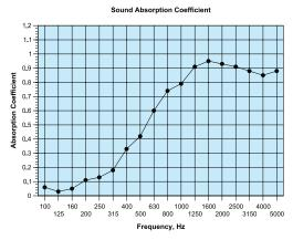
Calculated to EN ISO 11654:1997 ® 0.90, Calculated to ASTM C 423 - 01- NRC 0.55
