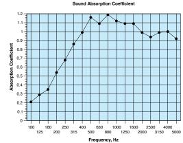
Calculated to EN ISO 11654:1997 ® 0.90, Calculated to ASTM C 423 - 01- NRC 1.0
