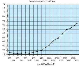
alculated to EN ISO 11654:1997 a 0.15, Calculated to ASTM 23 - 01 - NRC 0.20
