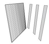
Mounting the panels over battens will increase performance to 0.45 NRC test have proven.
